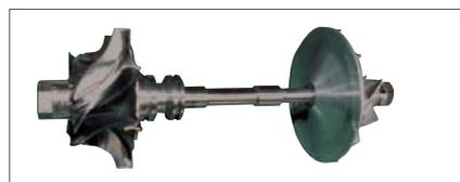
Fig 4: Turbocharger turbine
