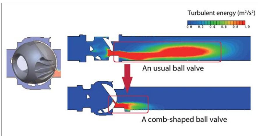
Figure 5: Comparison on analysis results between usual ball valve and comb-shaped ball valve
