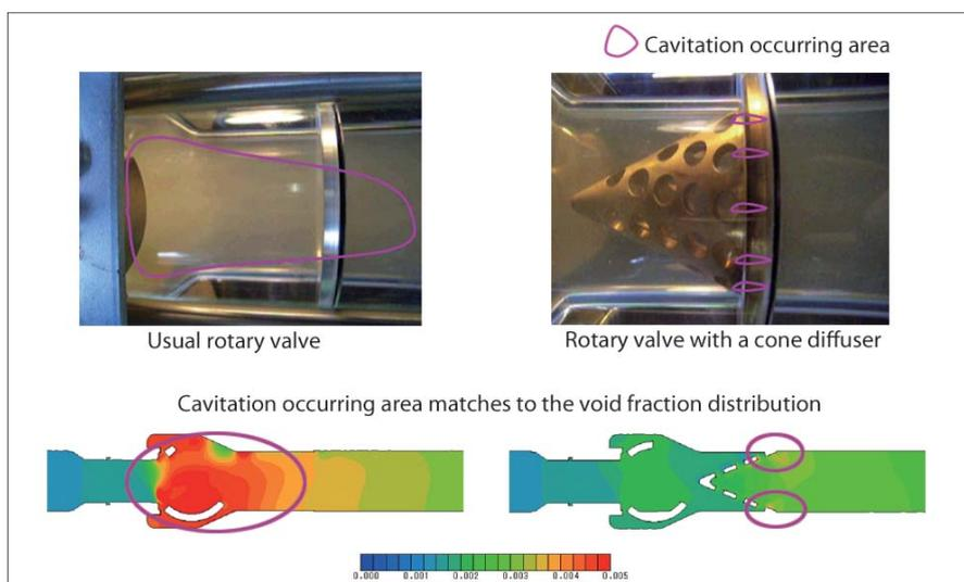
Figure 3: Cavitation experiment (above) and SC/Tetra analysis (below)
