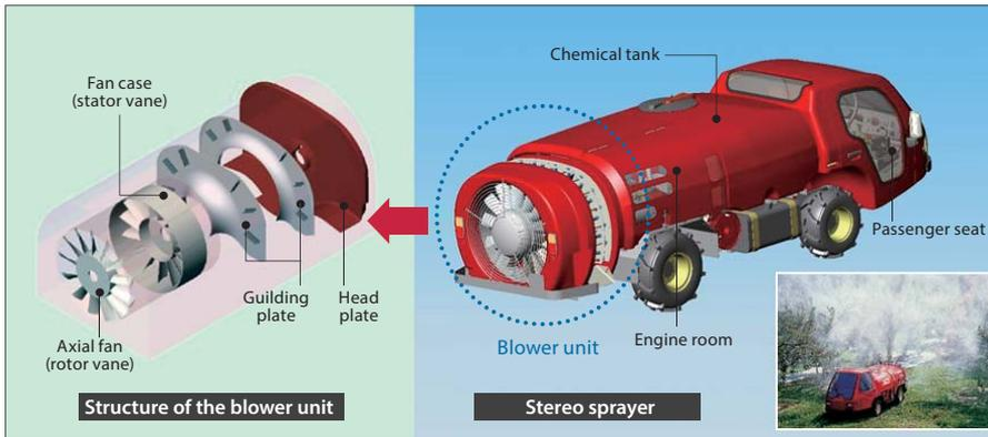
Figure 7: Stereo sprayer used for chemical distribution in orchards
