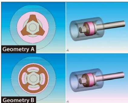
Figure 5: Examining two different geometries for the water suction seal within a pump
