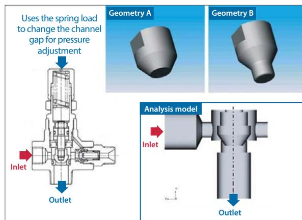
Figure 2: The evaluation on piston geometry on pressure control valve
