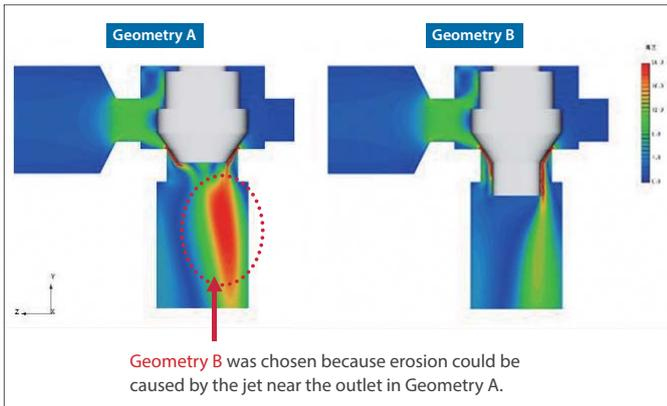
Figure 3: Simulation results of water velocity distribution around the valve
