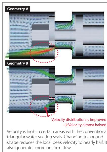
Figure 6: CFD analysis results (velocity distribution)
