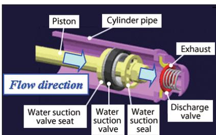
Figure 4: Structure of a pump with uniflow design
