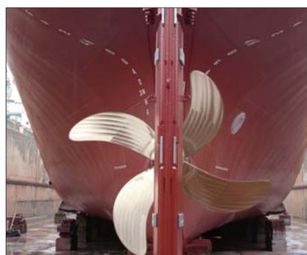
Picture 2: Propeller for chemical tanker
