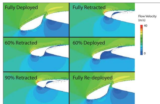
Figure 5: Velocity contours from FSI retraction/deployment analysis
