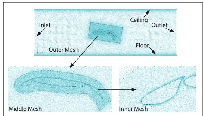
Figure 4: CFD model for Boeing-NASA CRM airfoil
